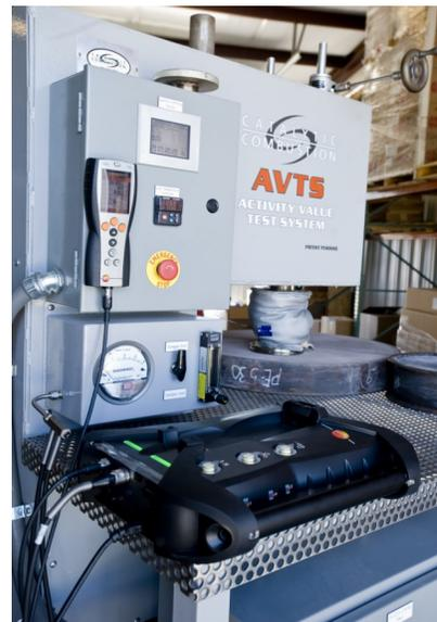
Chemical washing of catalysts is a proven method of extending the lifespan of a catalyst. However, there are circumstances where washing cannot restore sufficient activity to bring an engine into compliance. Up until now, the only way to know if a washed catalyst would work was to put it back into the housing and run a test. The risky trial-and-error process was costly in time, labor and lost production.
