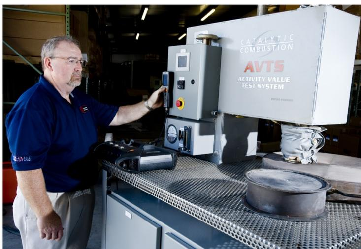
The overall process involves evaluating the catalyst in the condition it is received from the field, then washing it using CCC's exclusive 5-Step chemical cleaning system, and re-evaluating afterwards to see what improvement in the element's catalytic activity has been gained.
